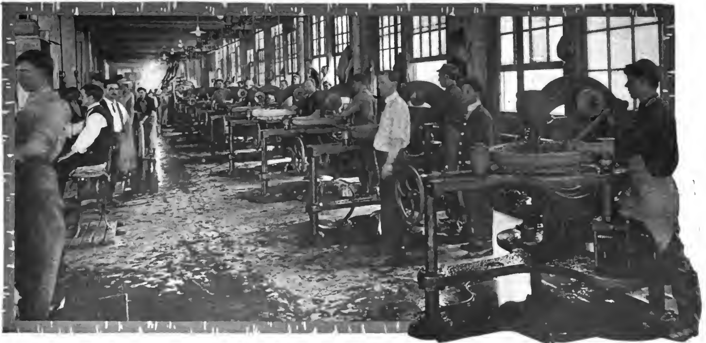
Part of the wrapping-room at the factory of the Goodyear Tire & Rubber Co., Akron, Ohio. In this room the tires are put through a wrapping process before going to the vulcanizer for their first cure
